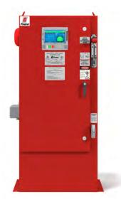
Description-Firetrol® FTA1800 Autotransformer Starting Fire Pump Controllers use an autotransformer to supply reduced voltage when starting the motor. The controller is of the closed circuit type where the motor circuit remains closed during the transition from start to run resulting in minimum line disturbance.
